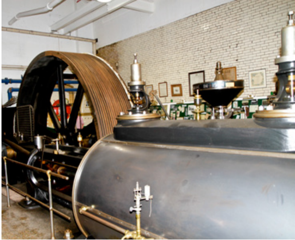
The enormous 18ft 6in wheel that used to drive everything in the Mill weighs 21 tons
