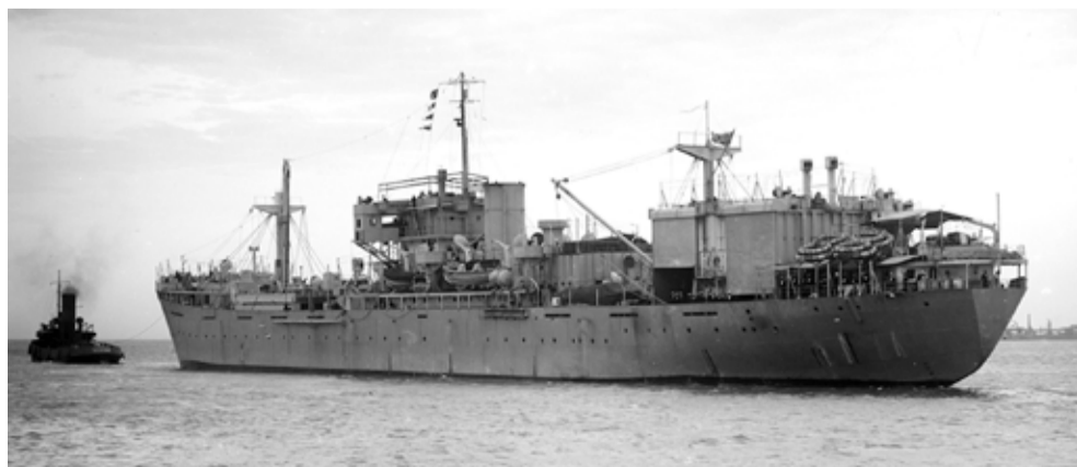
HMS 'Beaully Firth', sister-ship to HMS 'Solway Firth'. (Note the two aircraft engine test bays, one with shutter door partially open, located just forward of the poop)
